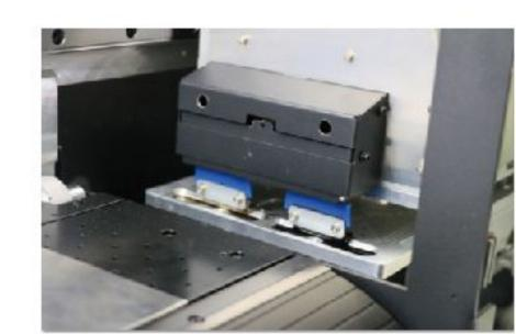
Automatic print head protection including anti-collision sensor, paper shortage sensor, provides multiple protections for the print head and improves the life of the print head.
