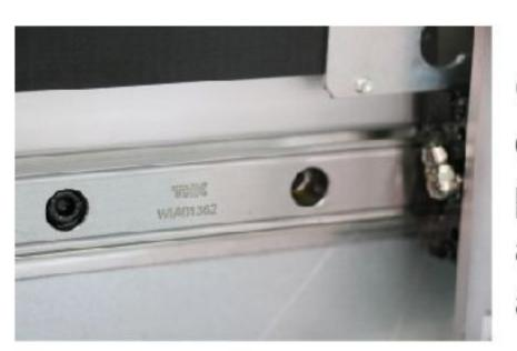
Genuine THK guide rail and other accessories ensure the precision requirements, such as parallelism and straightness accuracy of 0.001mm.
